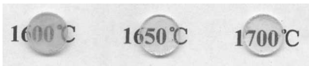
Fig. 11. Appearance of mirror-polished specimens sintered from 1600 to 1700 °C.
